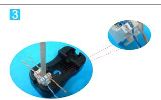
Follow the wiring sticker to place the wires into IDC slot. Keep the pairs twisted as possible as you can.
