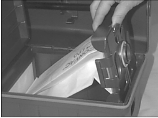
Fig 7. Refit the Retainer with Filter Bag attached.
