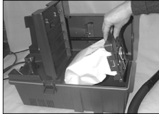
Fig 2. Remove the Filter Bag along with the Retainer from the Vacuum Cleaner.
